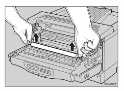
Insert the new transfer roller. When placing it, the green gear of the roller should be positioned on the left (1) as shown in the illustration.
