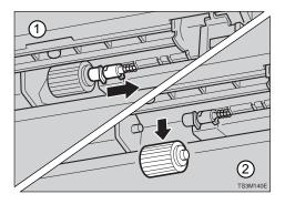
Set the new paper feed roller. While sliding the green lock lever to the right (①), set the new roller (②). After that, return the green lock lever to its original position (③).
