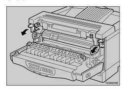
2 Slide the fusing unit toward you (①), and remove it from the printer (②) as shown in the illustration.
